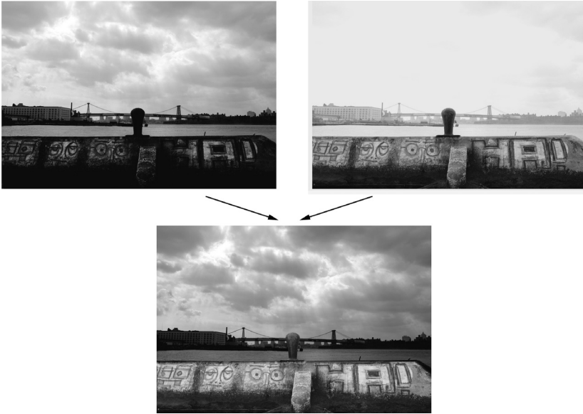
Figure 3.1 Merging of two digital images to increase dynamic range.
